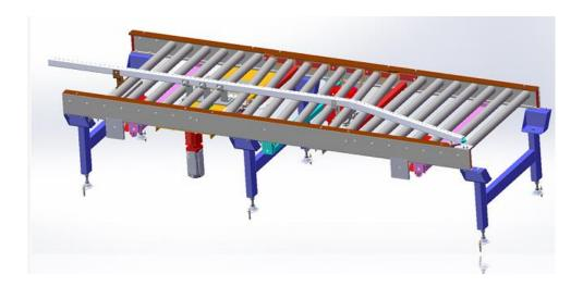
(3)The automatic turning over unit is generally arranged outside the shielded building, which is used for items requiring double-sided irradiation. After the first irradiation is completed, the automatic turning over unit turn over the item and then the second irradiation is performed. The automatic turning over unit generally adopts appropriate mechanical arm to complete turing over work.
