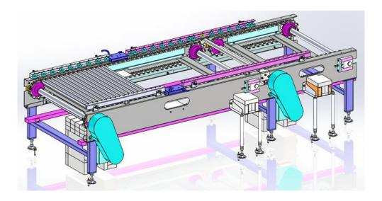
(2) The goods centering unit is arranged in front of the underbeam unit. By adjusting the center device on both sides of the transmission line, the article is forced to be centered in the middle of the transmission line when passing through this section, so as to ensure that the article is in the middle of the electron beam when receiving irradiation through the under beam unit, so as to ensure the utilization efficiency of the beam when the article irradiation.
